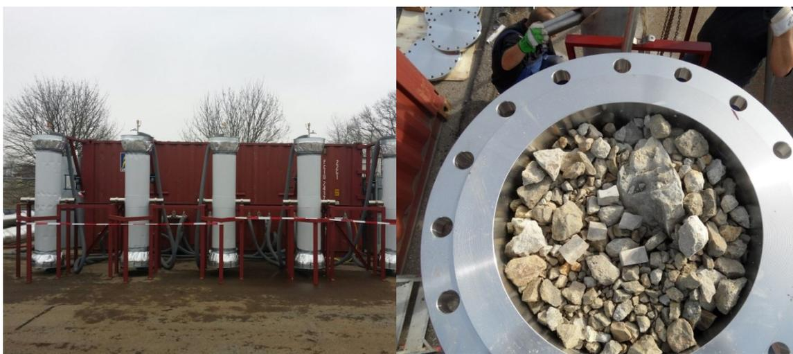
Fig. 2: (a) Bypass system in Kirschweidach and (b) Reaction columns while being set up
